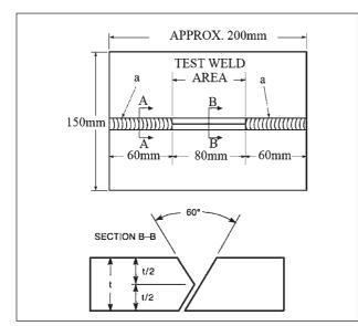
Figure 1 Oblique Y - groove test assembly, [7]
