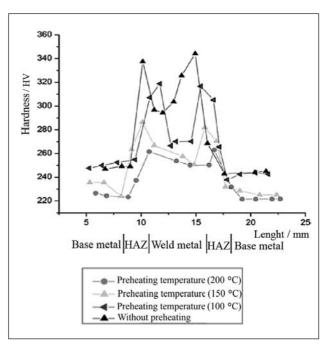
Figure 3 Hardness distribution for Y-probe (batch 180079, electrode T-80, Ø 4 mm)
