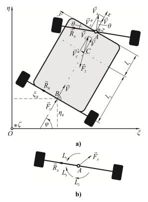
Figure 1. a) Simplified vehicle model; b) front axle.
