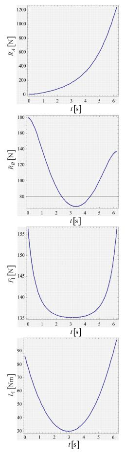
Figure 4. Reactions of constraints  $R_A(t)$ ,  $R_B(t)$ , and control forces  $F_1(t)$ ,  $L_1(t)$ .
