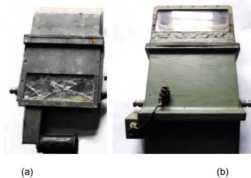
Figure 5. Types of Damages: mechanical (a); chemical (b)
