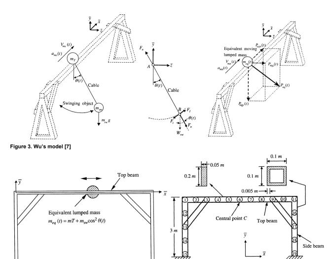
Figure 4. Wu's mathematical model for a crane hoisting a swinging mass [8]
