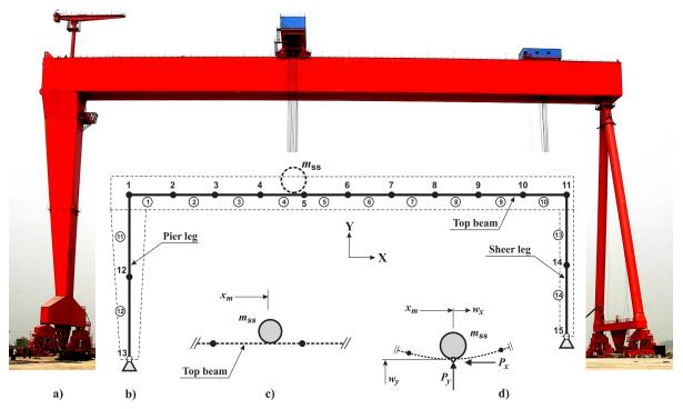
Figure 9. a) Real model of the gantry crane, b) FE model of the framework, c) Moving mass, d) Dynamic interaction [16]
