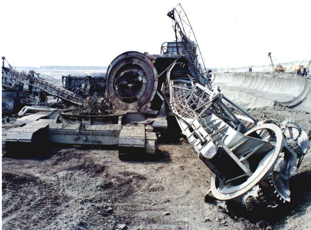
Figure 5. Failure of SRs 1200 bucket wheel excavator failure due to human error, /5/. Slika 5. Primer havarije rotornog bagera SRs 1200 usled ljudske greske, /5/
