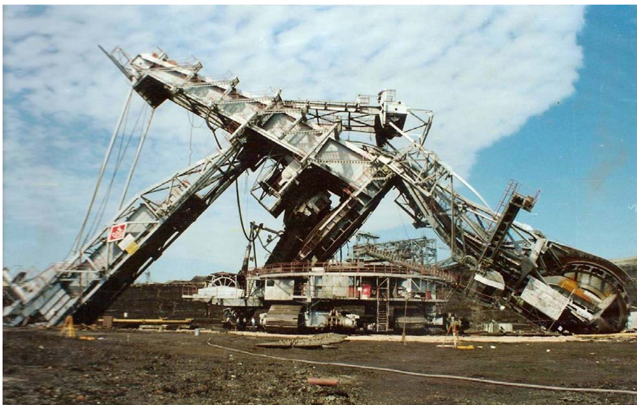
Figure 6. Failure of SchRs 630 bucket wheel excavator due to human error, /5/. Slika 6. Primer havarije rotornog bagera SchRs 630 usled ljudske greske, /5/
