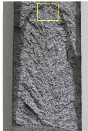
Figure 13. Final stretch zone after developed shear lips, prior to stable growth of ductile crack, corresponding to region CA in Fig. 3.
