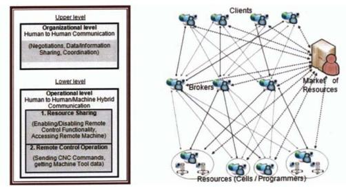
Figure 1. Multiplex communication system levels for remote control and network user communication channels (Putnik at al., 2011 and Shah at al., 2012)
