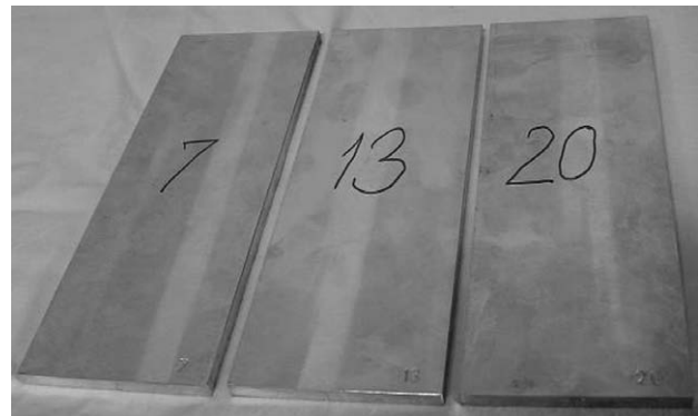
Figure 3: Thermally processed and machine prepared forged elements for FSW with the dimensions of 180 mm × 65 mm × 5 mm
