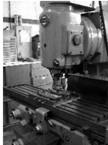
Figure 5: Tool for the friction-stir welding with a backing plate on water desk
