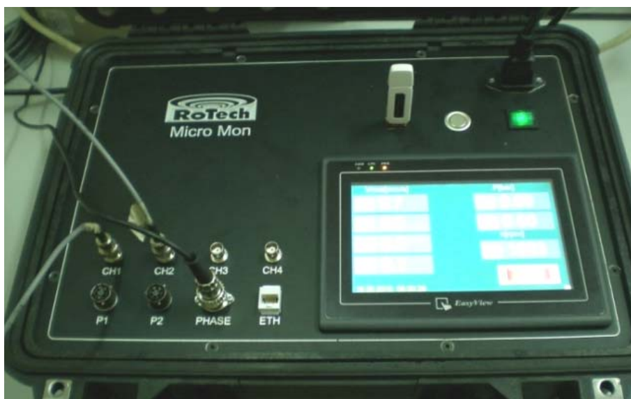
Figure 4. The general view of MicroMon portable device for vibrodiagnostics.
