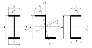
Figure 1. a) I-section; b) Z-section; c) Channel-section
