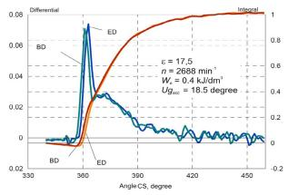
Figure 4. Integral and differential combustion rate for biodiesel and commercial diesel fuel at full load, for engine speed 2688 min<sup>-1</sup> [14, 15].
