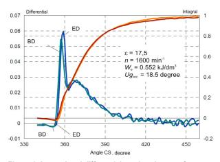
Figure 3. Integral and differential combustion rate for biodiesel and commercial diesel fuel at full load, for engine speed 1600 min<sup>-1</sup> [14, 15].
