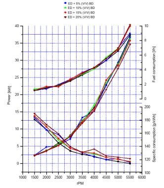
Figure 7: Comparative engine flat road load characteristics recorded for operation with ED and blends of ED and BD
