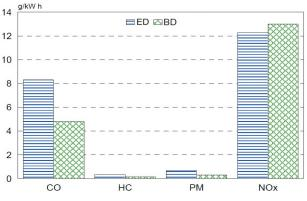
Figure 5. The values of emission of toxic components obtained by the European Steady-state Cycle (ESC), for engine operating with compression ratio of 17.5, with ED and BD [14, 15].
