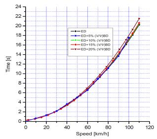
Figure 8. Vehicle acceleration from 0 to 100 km/h
