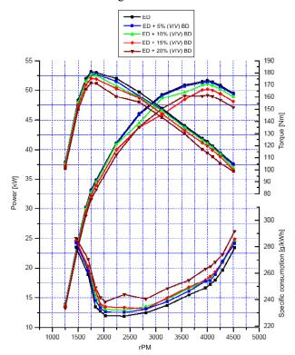
Figure 6: Diagram of engine full load characteristics recorded with ED and blends of ED and BD
