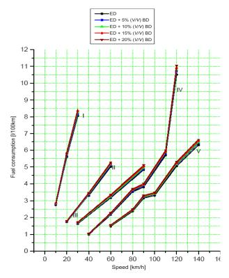
Figure 10. Fuel consumption of vehicle with ED and blends of ED and BD in all gears
