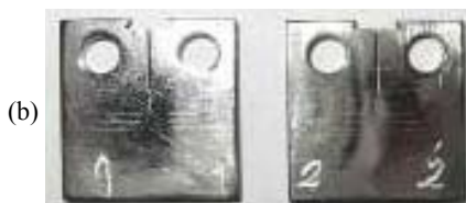
Figure 2. Modified CT specimen (a) and S316L specimens (b). Slika 2. Modifikovana CT epruveta (a) i S316L epruvete (b)
