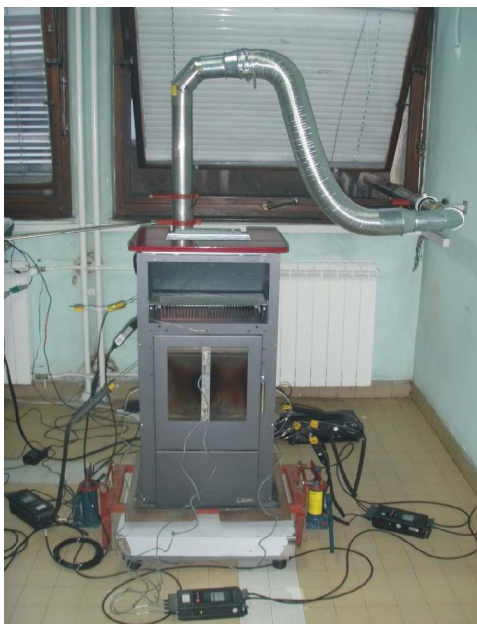
Figure 3. Pellet stove on the test installation
