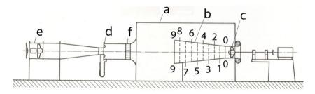
**Figure 1. Test bed for experimental diffuser flow research** (a) – reservoir, (b) – diffuser, (c) – axial fan impeller, (d) – flow meter, (e) – booster fan, (f) – honey-comb
