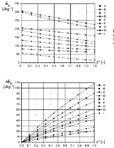
Figure 3. Swirl flow specific energy  $e_{s_i}$  along the diffuser  $(z^* = z/L)$  for the measuring series: A to I.
