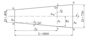
Figure 2. The main dimensions of the conical diffuser
