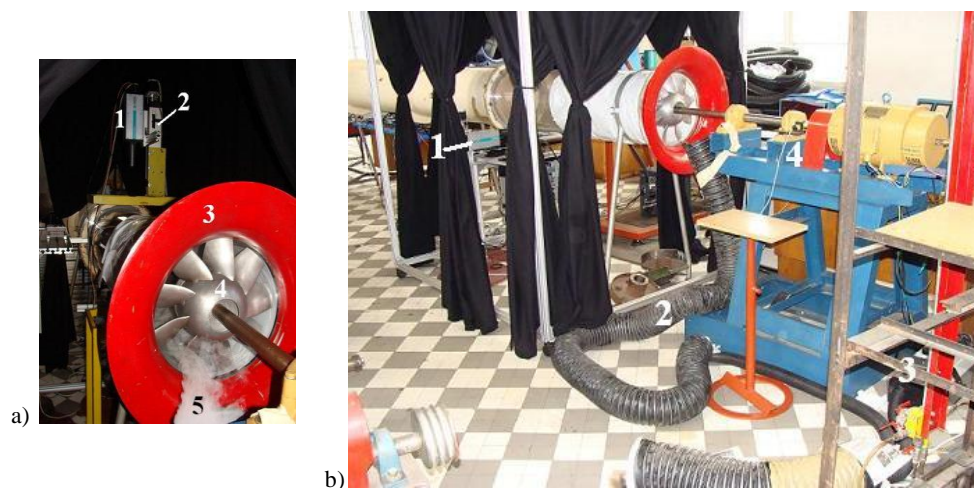
Figure 12. Test rig for LDA measurements
