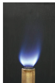
Slika 7. Fotografije plamena u slobodnom prostoru, nominalna snaga, 9 kW, S_2 = 1,13 , S_1 = 1,98 \lambda_2 = 1 , \lambda_1 = 1,2 . Figure 7. Typical image of the swirling flame, nominal power, 9 kW, S_2 = 1,13 , S_1 = 1,98 \lambda_2 = 1 , \lambda_1 = 1,2 .
