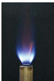
Slika 6. Fotografije plamena u slobodnom prostoru, nominalna snaga, 9 kW, S_2 = 0,73 , S_1 = 1,98 \lambda_2 = 1 , \lambda_1 = 1,2 . Figure 6. Typical image of the swirling flame, nominal power, 9 kW, S_2 = 0,73 , S_1 = 1,98 \lambda_2 = 1 , \lambda_1 = 1,2 .
