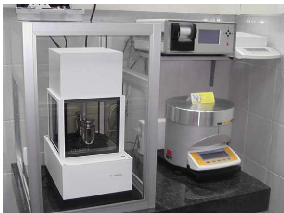
Fig. 7. Comparator Sartorius CCE1000 S-L and susceptometer
