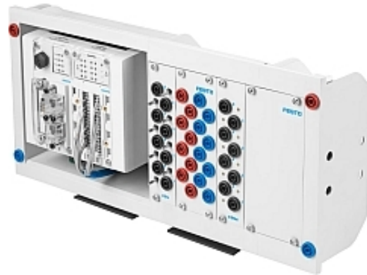
Figure 2. Festo PLC didactic module [6].
