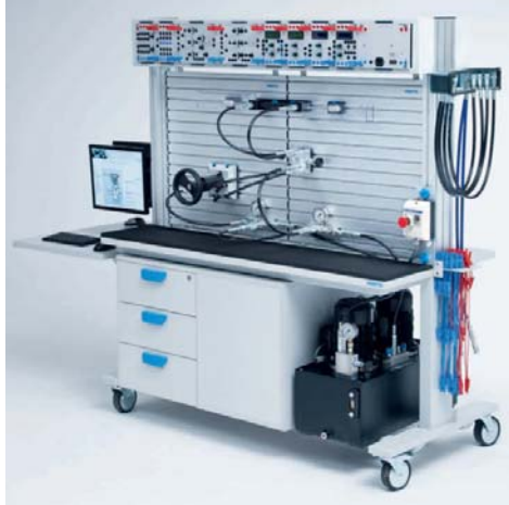
Figure 1. Example of didactic equipment for students basic training level in hydraulics [5].
