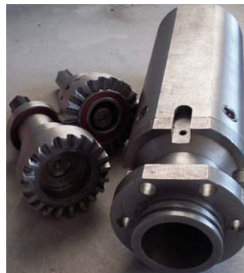
Figure 1. Coaxial reduction gear box with gear ratio i = 20
