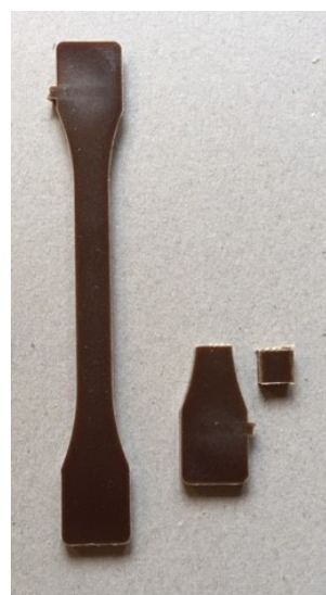
Figure 5 Pigment filled polymer (dog-bone shaped) sample (14.7 cm long, 2.0 cm wide at ends, 1.0 cm wide in the middle, 0.4 cm thick)
