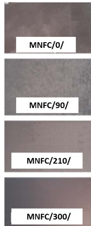
Fig. 2 Samples of cut-offs (60 x 15 mm 2 ) from MNFC films produced from pulp refined with different enzymatic pretreatment time (Table 1). Transparency and uniformity of films increases with hydrolysis time.
