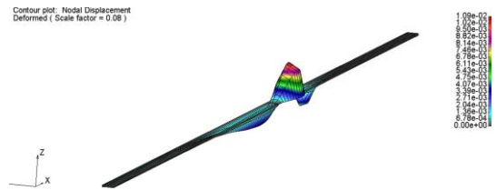
Figure 3: Air conduction response of the basilar membrane for excitation frequency of 1 kHz
