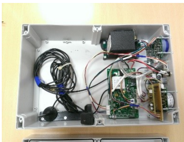
Figure 3. ekoNET device with low-cost electrochemical gas sensors
