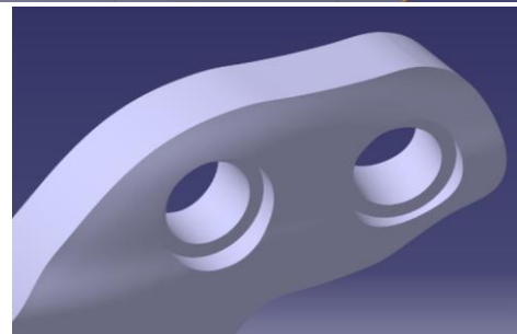
Figure 21. Creating screw holes
