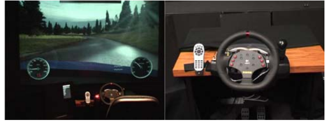
Figure 3. Driving simulator used for evaluation of spatial auditory interfaces and HDD [18]
