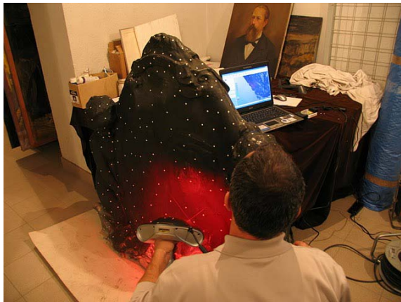
Figure 3. Laser scanning of the monument fragment
