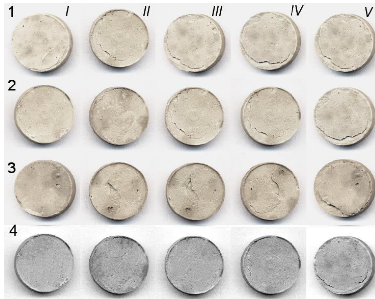
Fig 3. Surface of the samples IM-CrT10 (1), IM-CrT20 (2), IM-CrT30 (3), and IM-CQ (4) upon 0 (I), 30 (II), 60 (III), 90 (IV), and 120 (V) minutes long cavitation erosion.
