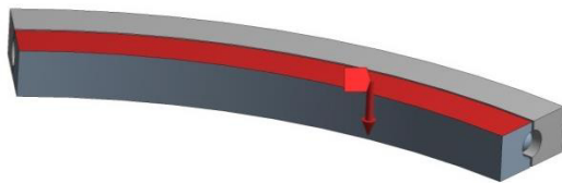
Fig. 10 Model of new slewing bearing solution for FEM
