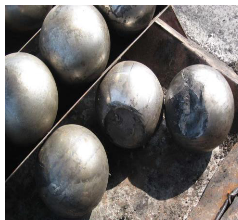
Fig. 12 Lost operation capacity of highest loaded ball
