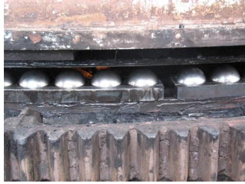
Fig. 3 Thrust ball bearing with classical pivot arrangement
