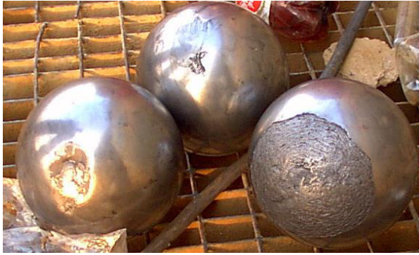
Fig. 13 False brinelling and flaking of loaded balls
