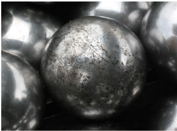
Fig. 14 Abrasive wear of ball on contact surface
