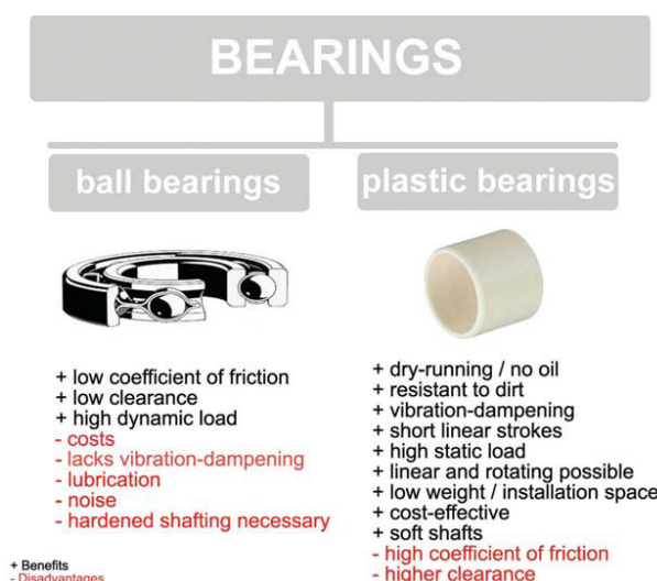
Figure 3. Comparing ball bearings to plastic bearings
