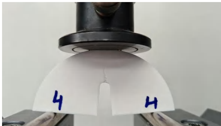
Fig. 1. Three point bending test of PETG SCB specimen with radius 40 mm and notch radius 2.2 mm
