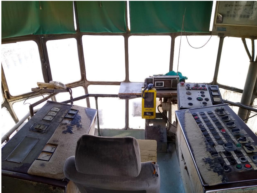
Figure 2. Control cabin of SRs 1200x24 /4 bucket-wheel excavator.
