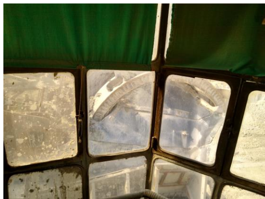
Figure 4. The exterior glass surfaces of the operator's cab are not equipped with wipers to clean them.
