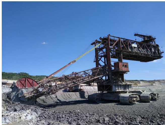
Figure 1. Bucket-wheel excavator SRs 1200x24/4.
