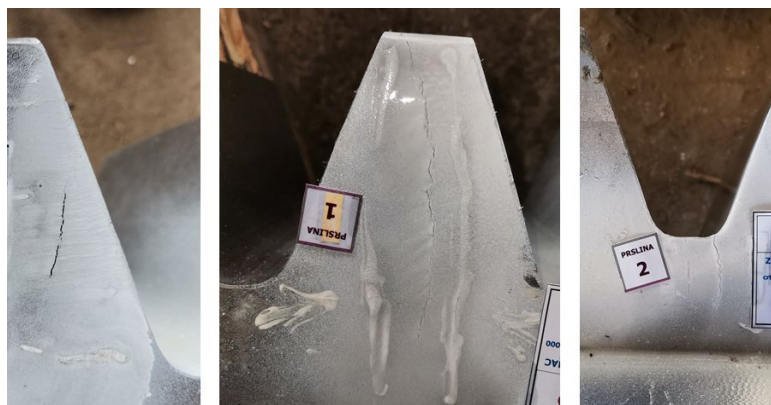
Figure 1. Examples of observed defects on gear ring of a bucket-wheel excavator.
