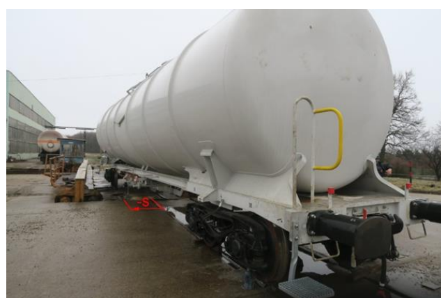
Figure 9: Transfer table displacement to simulate rotation angle \psi < -5.16^\circ [5]
