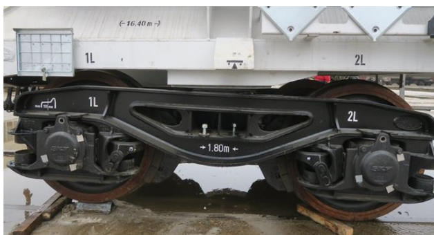
Figure 6: Rotation in the vertical plane bogie vs. car body for an angle \alpha - \varphi = +2.3^\circ [5]
