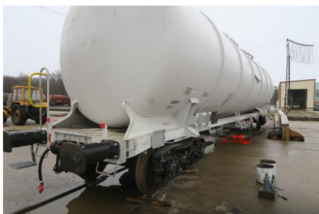
Figure 8: Transfer table displacement to simulate rotation angle \psi > 5.16^\circ [5]
