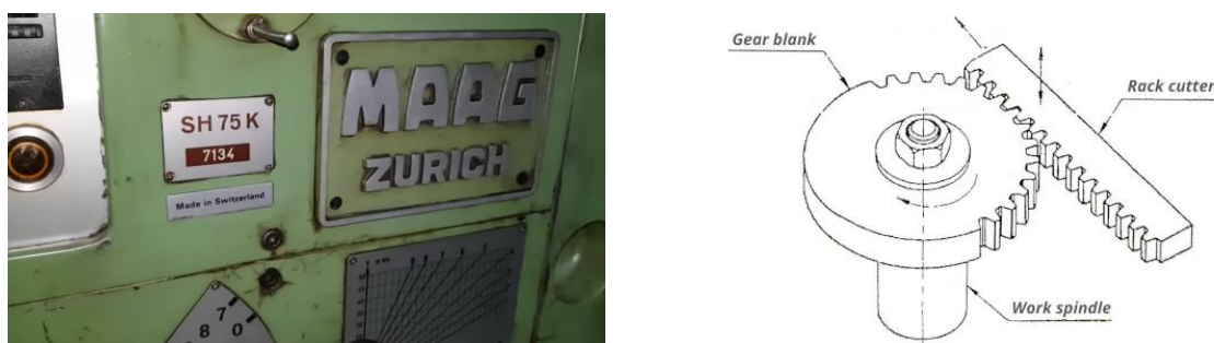
Fig. 6. MAAG gear shaper model designation (SH 75 K) [9] and MAAG method scheme [10]
