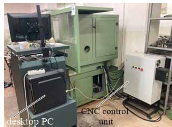
Figure 9. Representation of a built 3+2-axis grinder – Profiator 100 (back side view)
