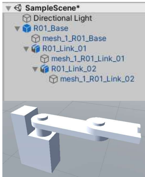
Figure 3. Design tree and 3D model of SCARA robot in Unity
