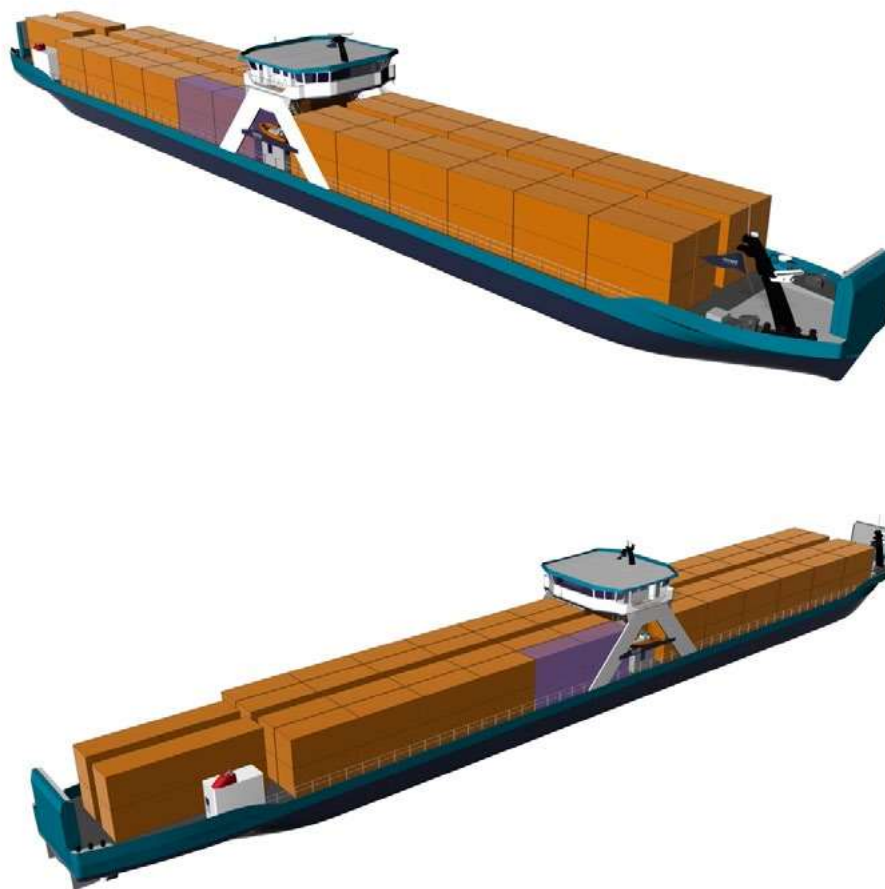
Figure 12. Concept of the double-end access container Ro-Ro vessel for the Vessel Train
