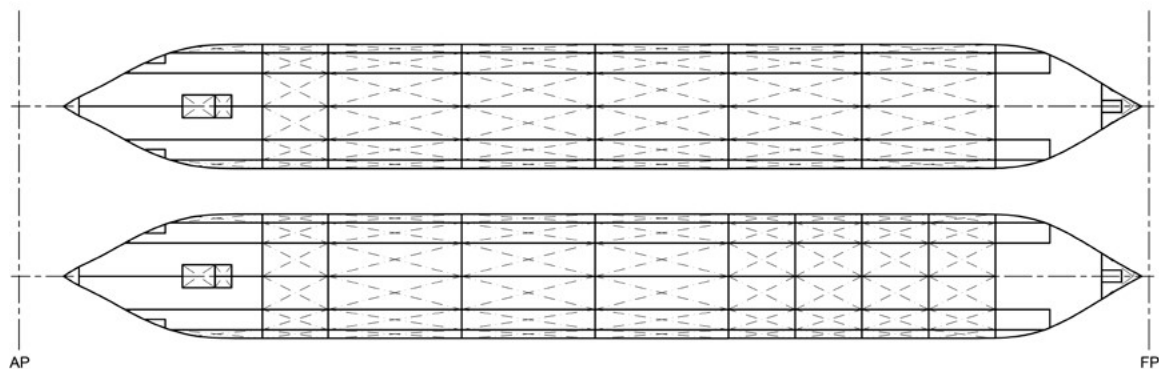
Figure 10. Original (upper image) and modified (lower image) subdivision of the stern access concept
