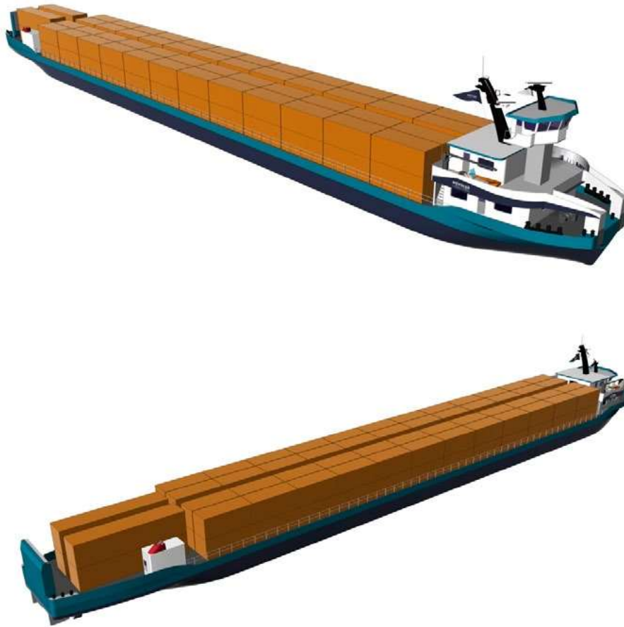
Figure 13. Concept of the stern access container Ro-Ro vessel for the Vessel Train
