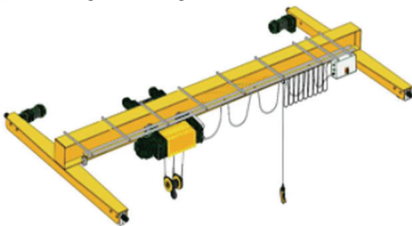
Fig. 1. Single Girder Bridge Crane
