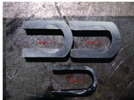
Fig.9. U shaped securing elements after testing
