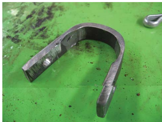
Fig.3. Deformed U-shaped securing element
