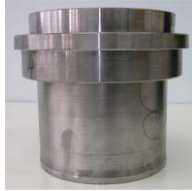
Fig. 6. Deformed sample – shrinking absorber
