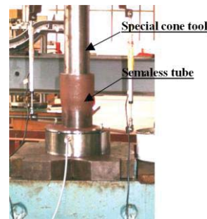
Fig. 4. Working principles – expanding absorber
