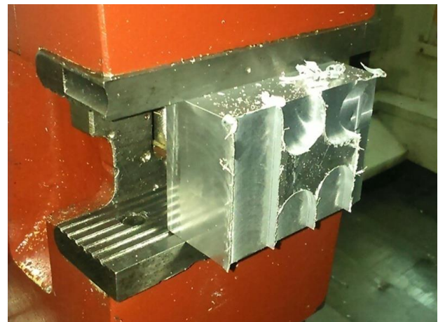
Figure 4. Workpiece after rough machining [7]
