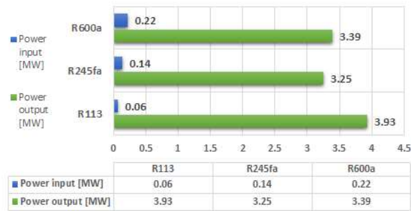
Fig.3. Turbine power output and feed pump power input for R113, R245fa and R600a, [MW]
