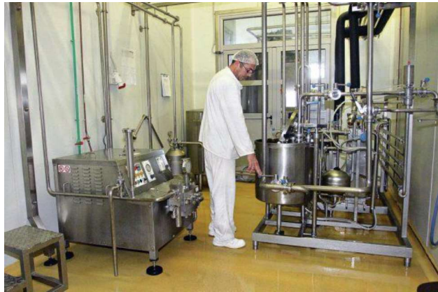
Figure 3. Part of the dairy production plant - line for thermal processing of milk
