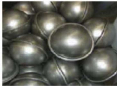
Figure 14 PCM encapsulated in metal balls 26.
