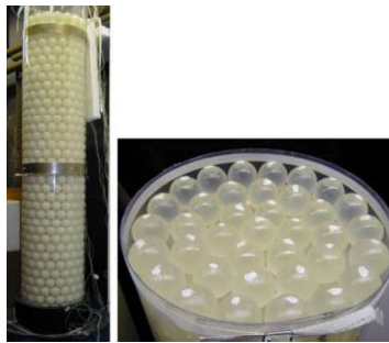
Figure 13 PCM encapsulated in spheres 26.
