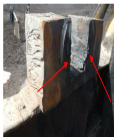
e) Damage at the carrying structure of an embedding of the stacker conveyor rejecting drum – side view;
