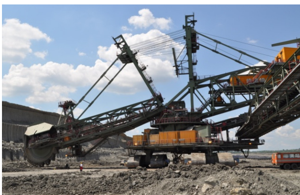
Figure 1. BWE SchRs 1600 in operating conditions: mass (with mobile conveyor) 3345t, theoretical capacity 6600m 3 /h
