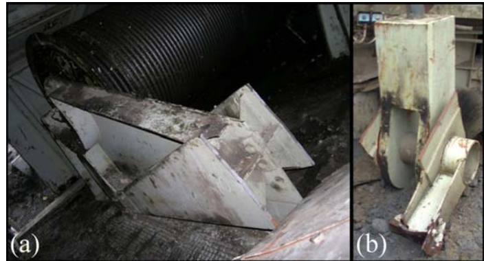
Picture 3. – 3D model and the broken-down support of the right portal tie-rod [13]
