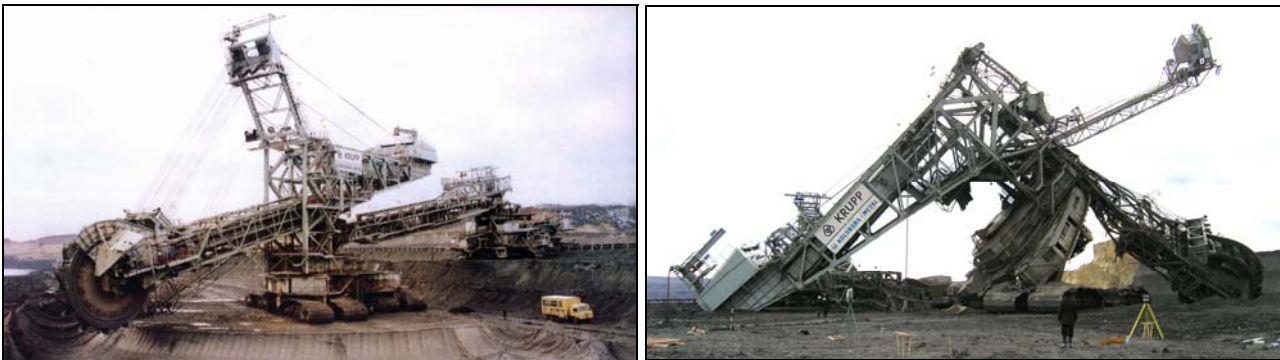
Picture 2. – BWE SchRs 1760 before and after the collapse [14]
