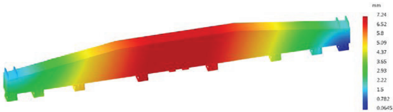
Figure 11: Traverse displacement field
