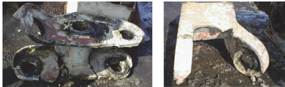
Fig. 6 Typical failure of the TWB structure
