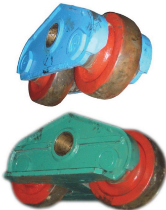
Fig. 7 Original and redesigned TWB structure
