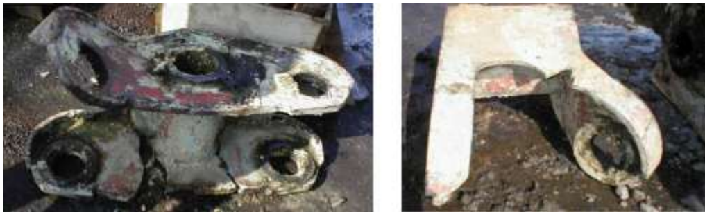
Figure 13: Typical failure of the TWB structure [14]
