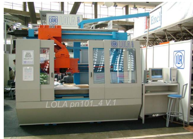
Figure 11. Vertical 3-axis parallel kinematics milling machine
