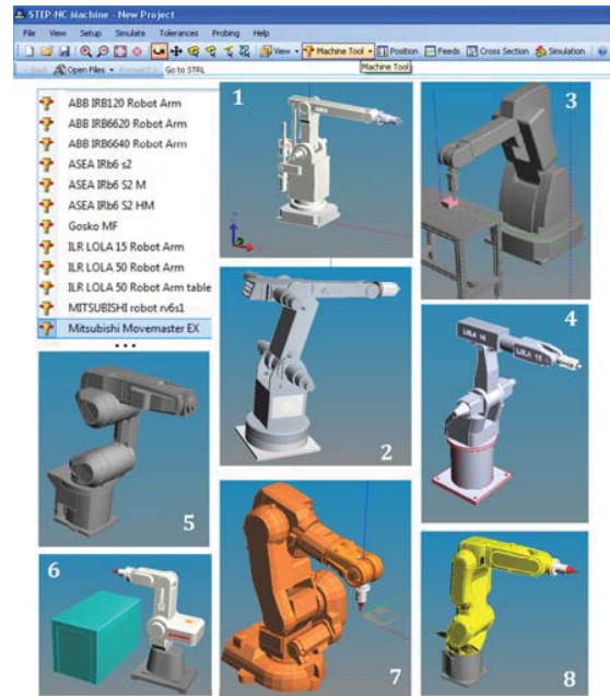
Fig. 8. Example of configured virtual robots for machined in STEP-NC Machine
