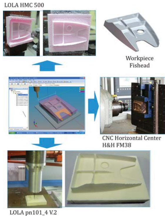
Fig. 18. Examples of mill machining based on STEP-NC
