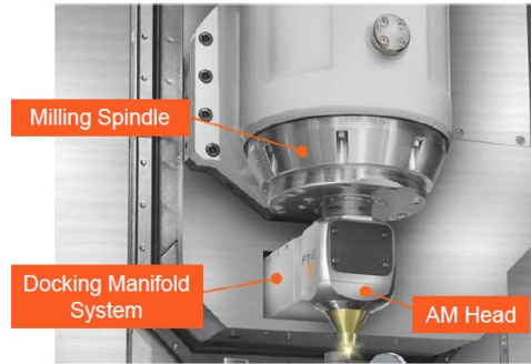
Figure 11. AM head and milling spindle in same machine [19,37]
