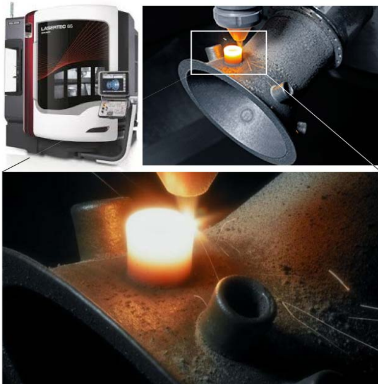
Figure 12. 3D printing and 5-Axis machining combined in one machine [35]
