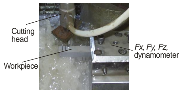
Fig. 5. Workpiece in dynamometer during experimental research [7]
