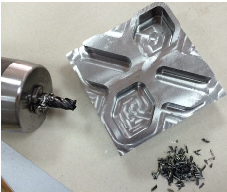
Fig.10 The cutting tool and chips
