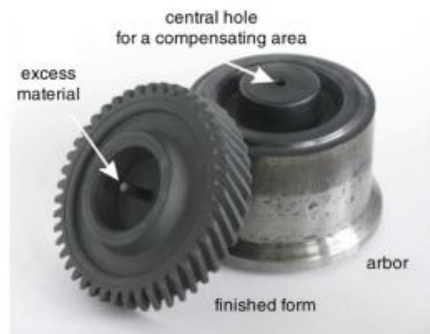
Fig. 5. Tool sided volume compensation for the gear forging [11]
