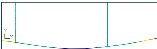
Fig. 6 Third natural frequencies of the test spindle
