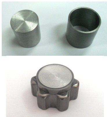
Fig. 11. Disassembled Al/Steel billet and workpiece after radial extrusion
