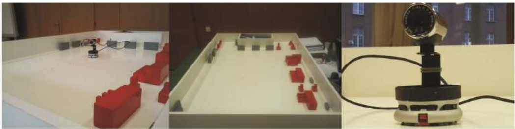
Fig. 1. The laboratory model of a manufacturing environment and the mobile robot Khepera II with USB camera
