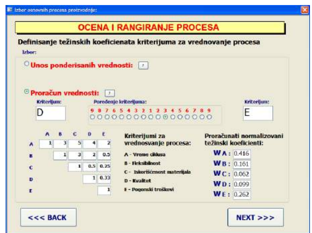
Fig. 6. Calculation of weights for the evaluation of alternative process solutions - the method (b)
