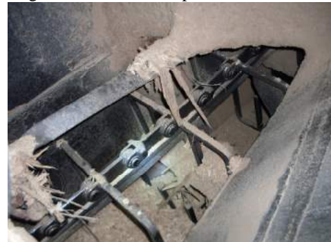
Fig. 1. Chain conveyor for raw wood chip
