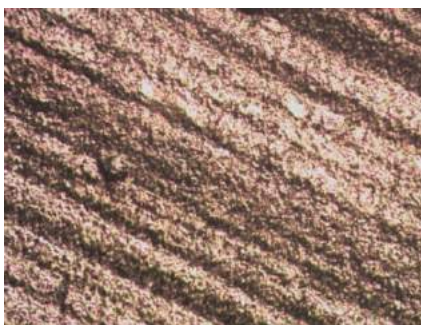
Fig. 5. Morphology of chromium coating
