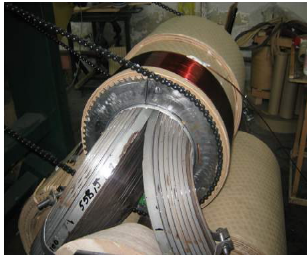
Fig.2. Technology of making the active part of a delta wound core transformer
