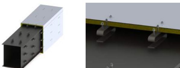
Fig. 6. Technical solution of conveyor light lining
