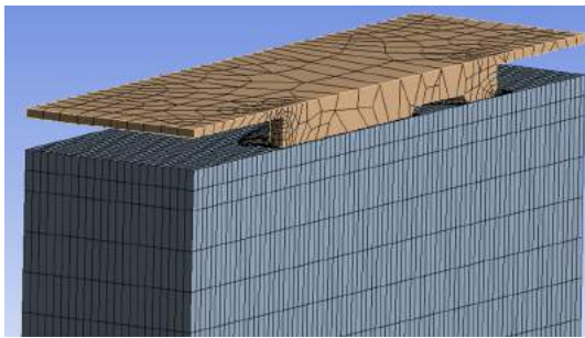
Fig.10. FE mesh used in analysis of symmetrical model of the rib forming using rubber pad
