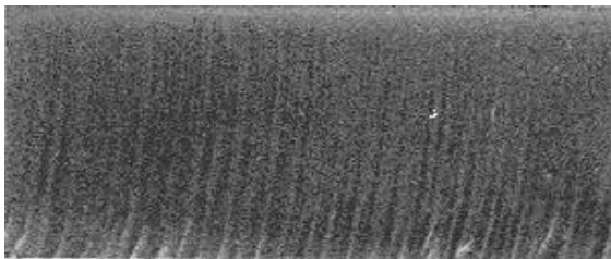
Fig. 2. Appearance of the surface machined with abrasive water jet
