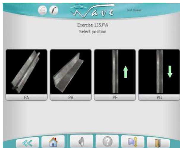
Fig. 5 Selection of welding position
