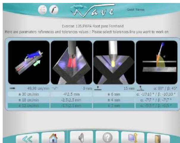
Fig. 6 Welding parameters determination
