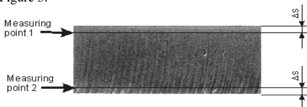
Fig. 3. Measuring points for the measurement of surface roughness
