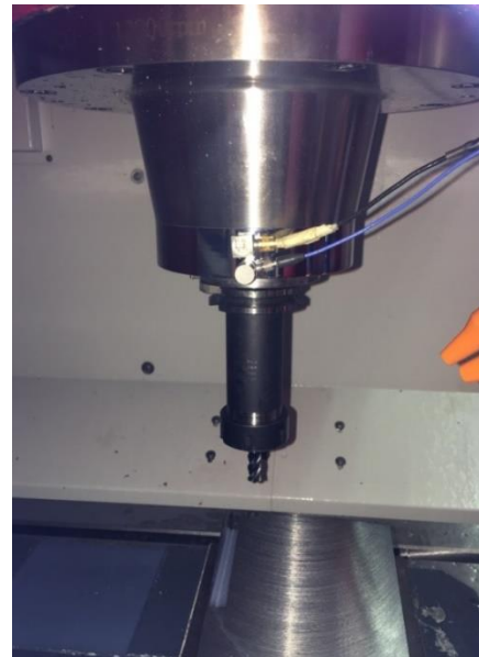
Figure 11. Machining of a 42CrMo4 workpiece at the EMCO ConceptMill 450 machining center
