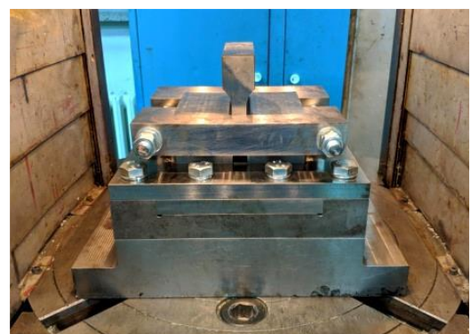
Figure 11. Plane strain die: (a) cross-section of the CAD model, (b) a photo of the die attached on the hydraulic press [17]
