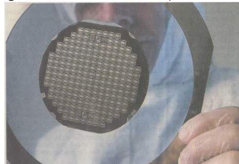
Figure 24. Separation of the chips from a silicon substrate by laser scribing (Philips, Netherlands)
