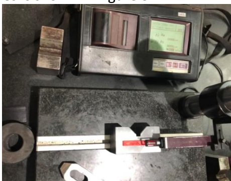
Figure 5. Surface roughness measuring point
