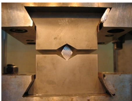
Figure 6. Upsetting by V-shape dies [16]
