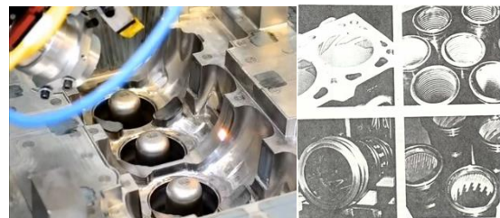
Figure 21. Cylinder bushings for diesel engines with hardening (MAN, German)
